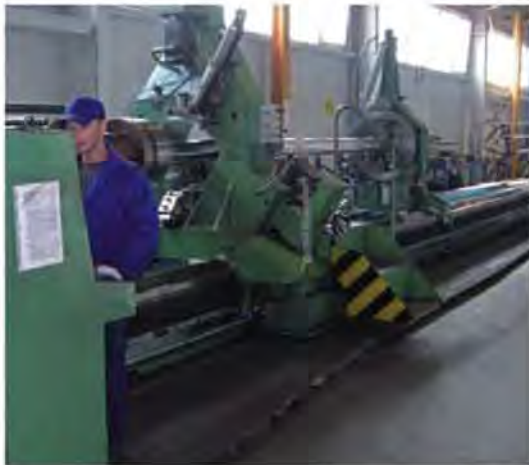
⌘ Machine for rolling aluminium cones
