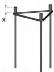
Reinforcement basket Z-0
