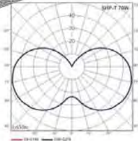
OS-1 S-70W, white diffuser - photometric distribution curve
