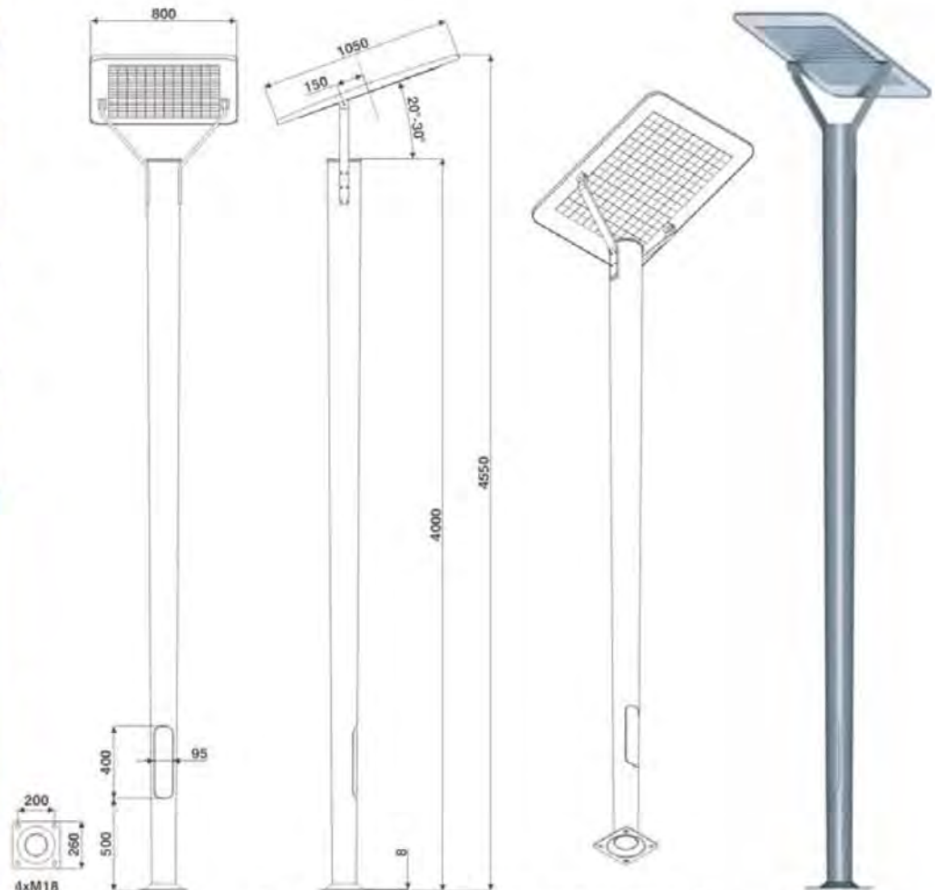
Reflector angle inclination 20° or 30° insulation class I IP65
