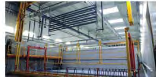
Columns on jig after anodizing process
