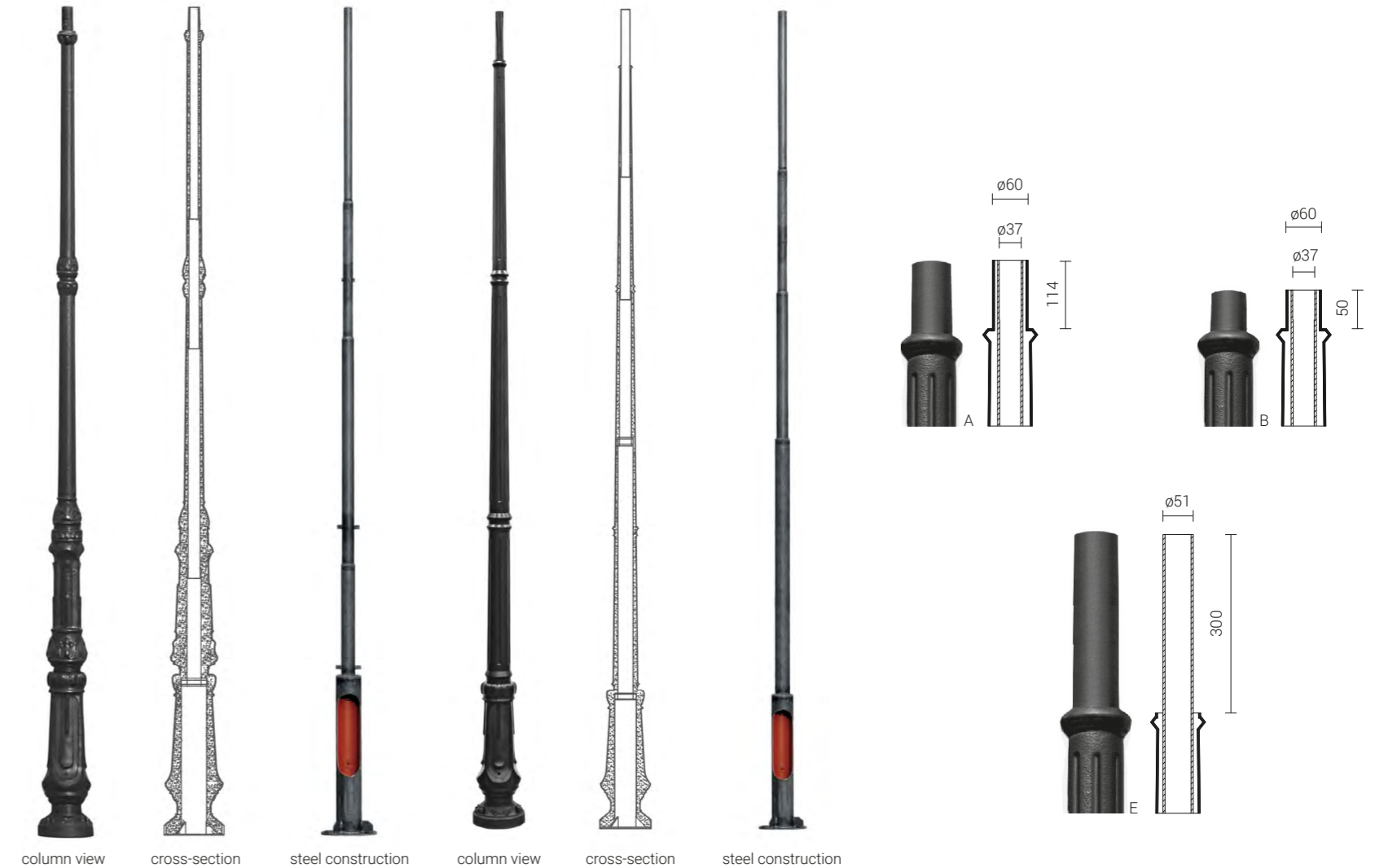
Cross-section of spigots in plastic coated poles
