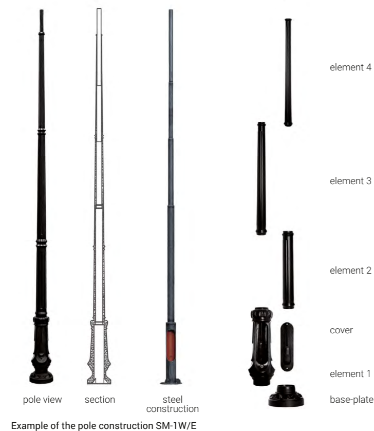
Example of the pole construction SM-1W/E
