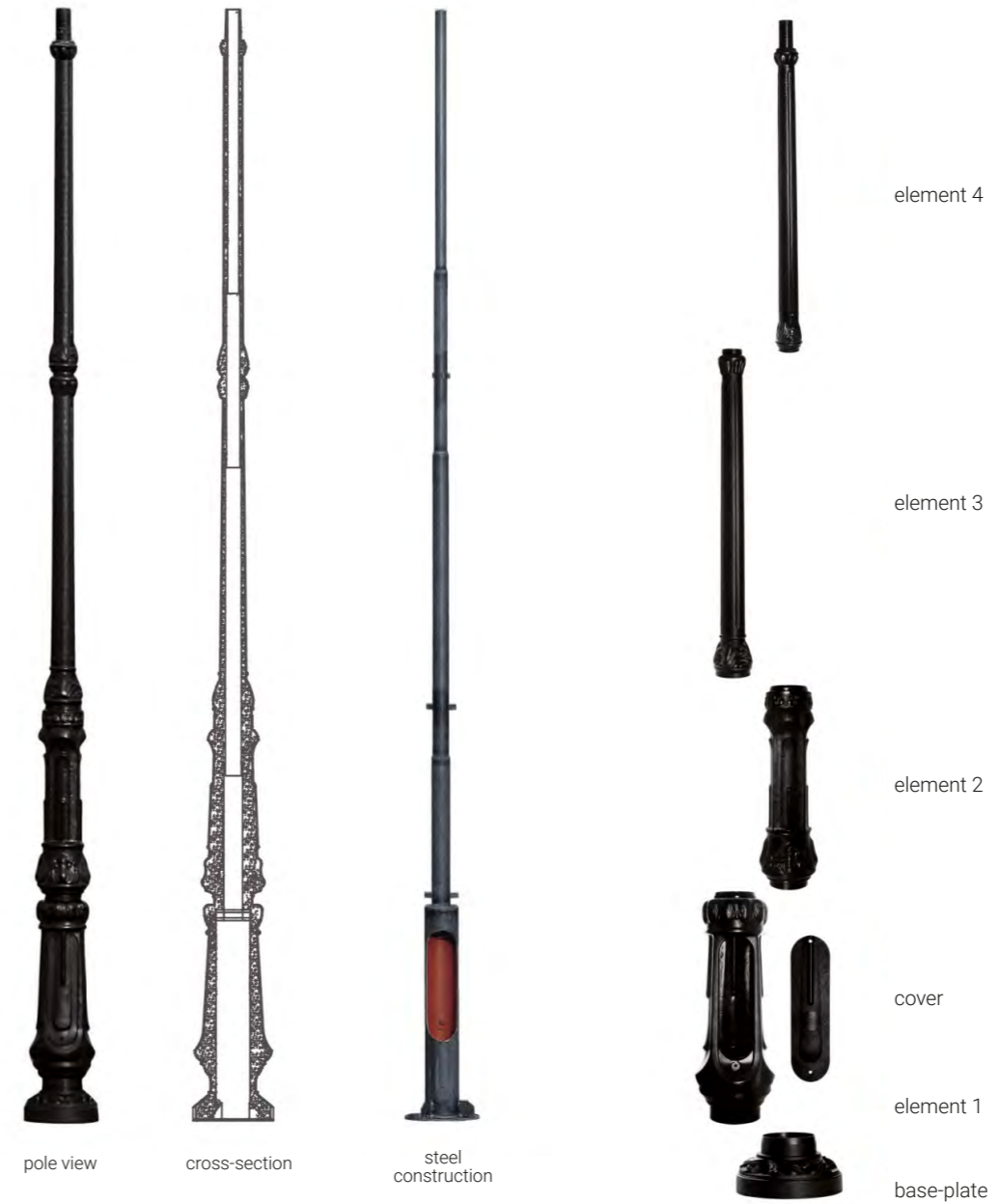
Example of the pole construction S-40W
