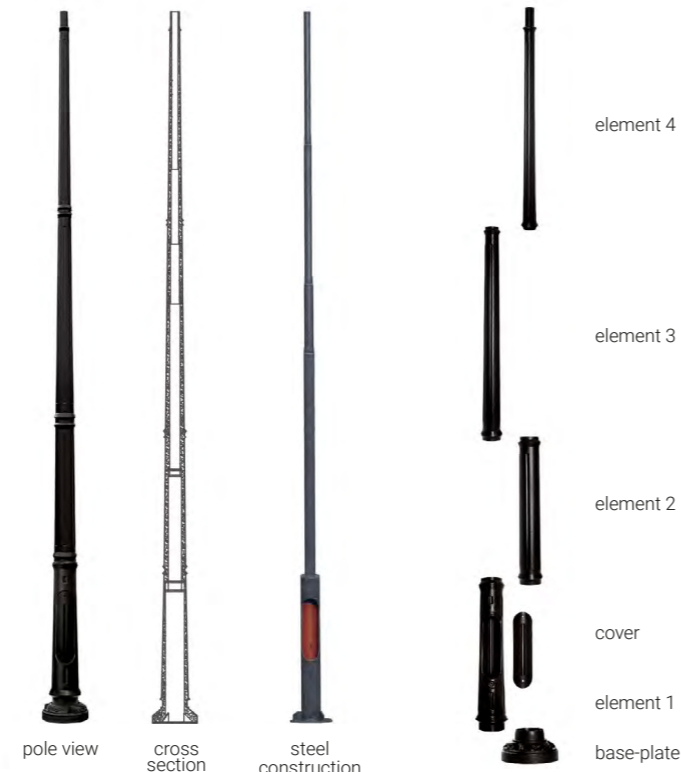
Example of the pole construction SP-4W
