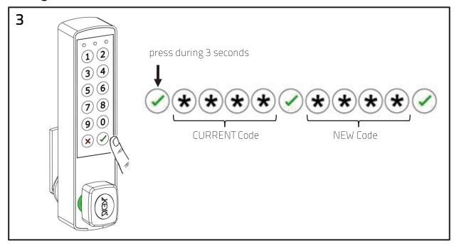
Press Enter key during 3 seconds. Introduce Current code and press Enter. Introduce New code and press Enter.
