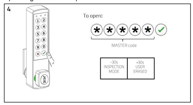
INSPECTION MODE Introduce Master code and press Enter. Close the lock by pressing Enter before 30s. The User code is not deleted. DELETE USER CODE
