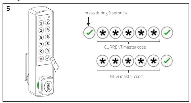
Press Enter during 3 seconds. Introduce Current code and press Enter. Introduce New code and press Enter.
