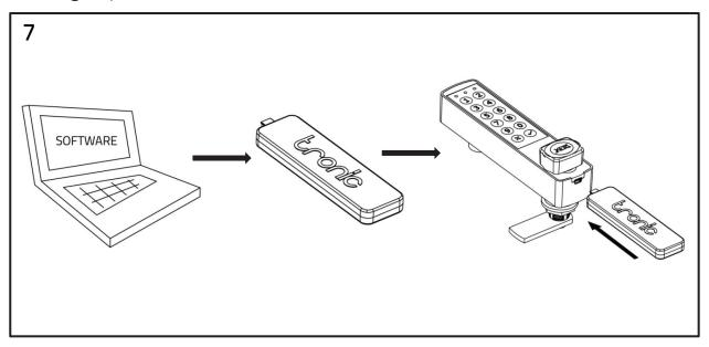
Load settings from the computer to the settings key (BLACK). Connect settings key to the lock.
